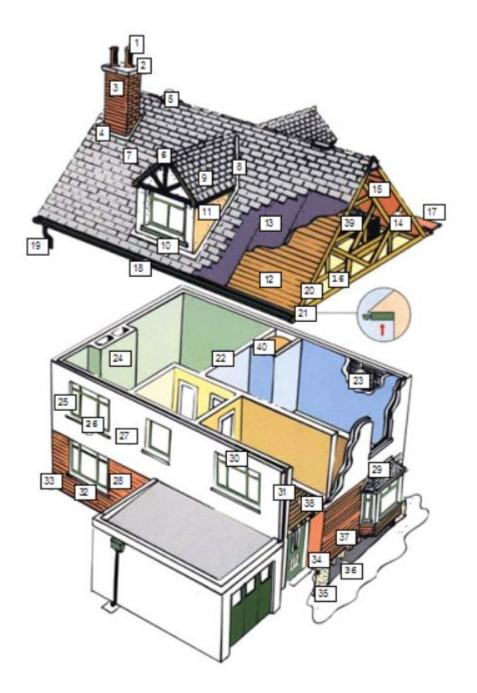
3 Chimney head Flashing 4 Ridge ventilation 5 Ridge board Slates/tiles 8 Valley guttering 9 Dormer projection Dormer flashing 10 Dormer cheeks 11 12 Sarking Roof felt 13 Trusses 14 15 Collar 16 Insulation 17 Parapet gutter Eaves guttering 18 Rainwater downpipe 19 20 Verge boards / skews 21 Soffit boards 22 Partition wall Lath / plaster 23 24 Chimney breast 25 Window pointing Window sills 26
